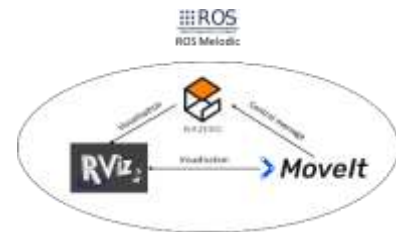
Figure 2 Structure of simulation environment
